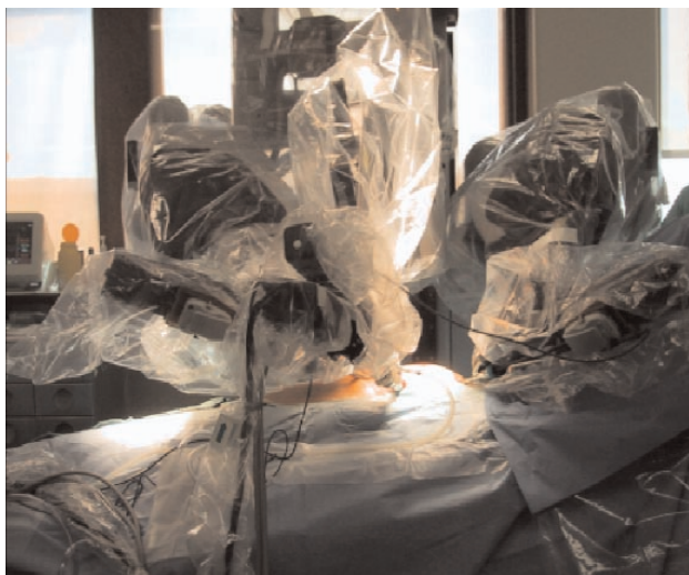
Figure 2. Patient-side surgical-arm component of the da Vinci telemanipulator.
