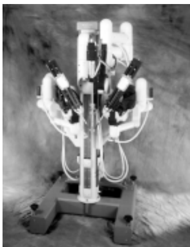
Figure 1. The Da Vinci surgical cart, with a central camera arm and two lateral instrument arms.
