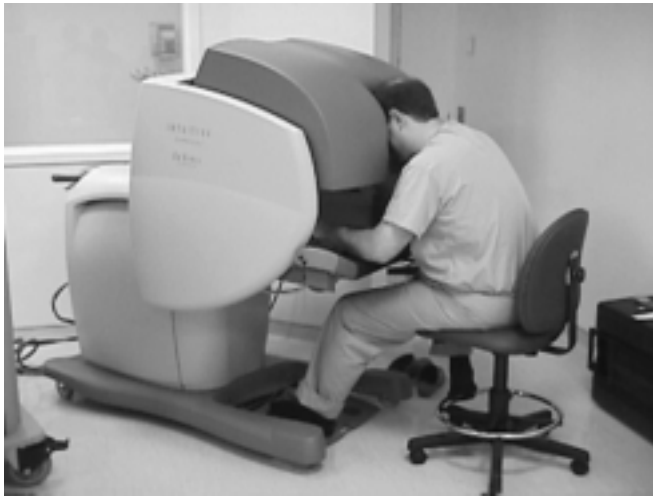
Figure 2. The Da Vinci surgeon's console, from which the robotic camera and instrument arms are controlled.
