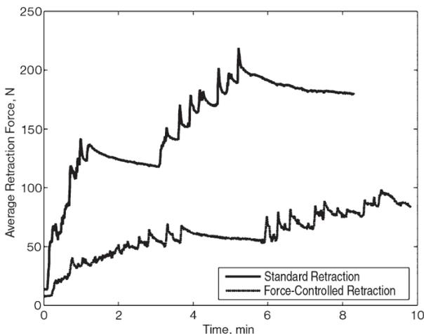
Figure 2. Comparison of retraction forces for a force-controlled sternotomy and a standard sternotomy, performed on 2 animals with similar weights.
