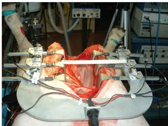
Figure 1. A novel instrumented retractor to enable real-time force monitoring during surgical retraction was used in the performance of standard median sternotomies in sheep placed in a supine position.
